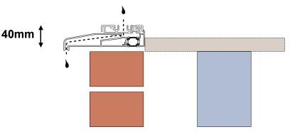
4) Standard Threshold with 150mm Cill (Open Out)
